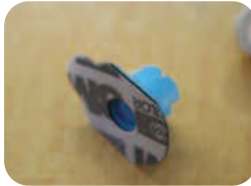
2. Apply 3M LeapIII (24mm) pad on lens cup. - 26mm pad is not recommended - lens cup must be plastic type
